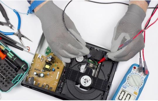
Gloves and finger cots with static control properties are made of (or treated with) materials that are inherently anti-static or static dissipative or blended with conductive materials. The ANSI / ESD SP15.1 is the standard of reference for In-Use Resistance Testing Of Gloves And Finger Cots. It covers multiple resistivity tests, including:
